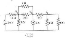
b) Find the load resistance for maximum power across it as shown in fig. What is the maximum power?
